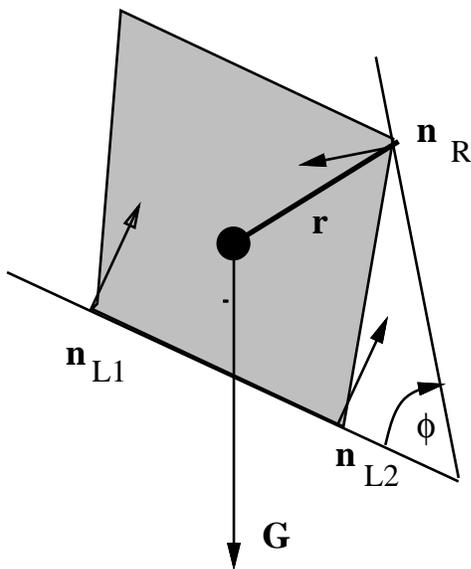
Figure 7.5: Contact normals and gravity vector in realspace.
