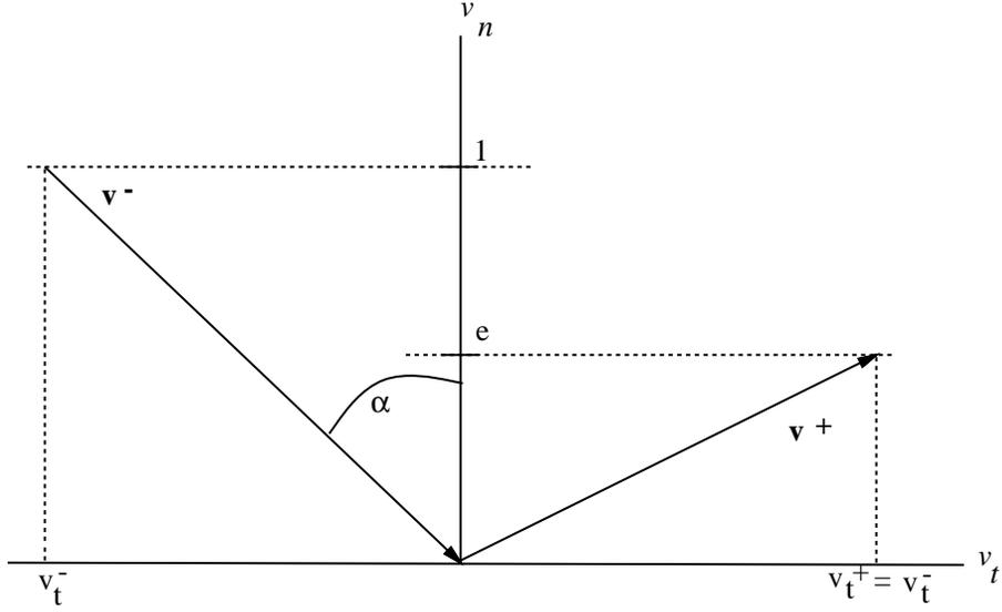
Figure 6.3:  $\mathbf{v}^\perp$  and  $\mathbf{v}^+$  in configuration space
