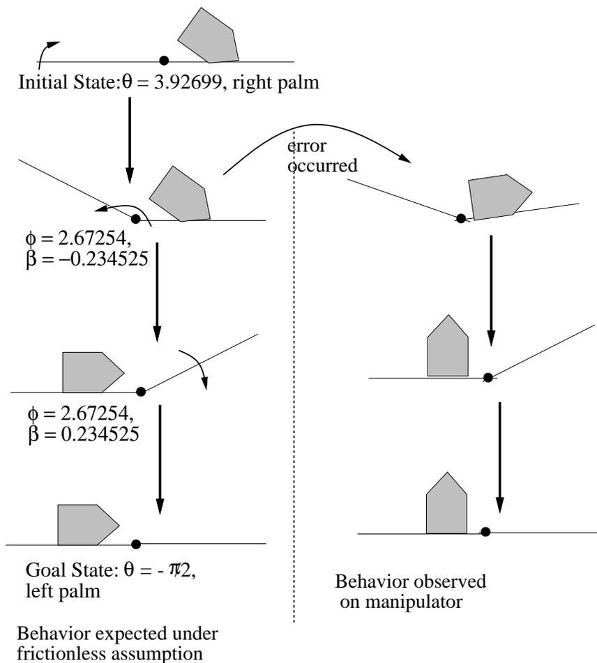
Figure 3.11: A plan which tended to fail.
