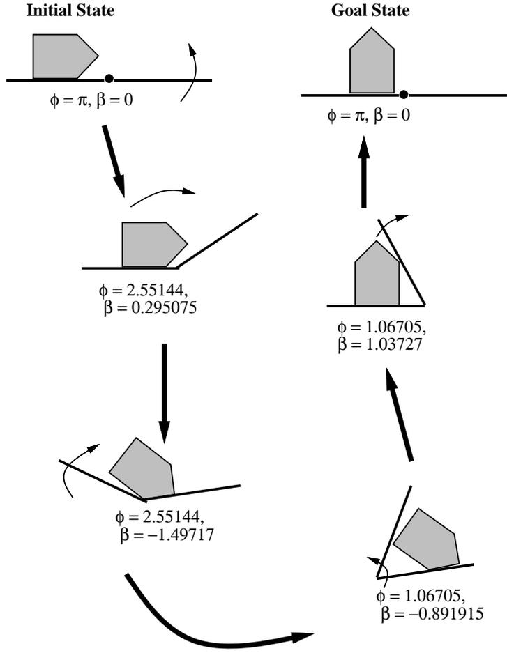
Figure 3.9: Example reorientation: from  $\theta = -\pi/2$  on left palm to  $\theta = 0$  on left palm
